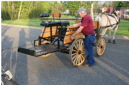
Hill Carriage Works in Buffalo, MN. The vehicle has a hydraulic lift in the back which is used to lift a person in a wheel chair into the carriage. The horse that is used is Olaf, Orphy and
